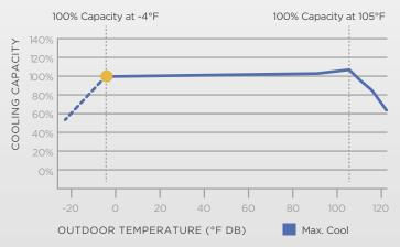
\* MLA018S4S-1P max cool performance indicated; Data illustrated to -4°F but unit effectively operates to -22°F (indicated by dotted line); 80°F db / 67°F wb entering indoor unit.
