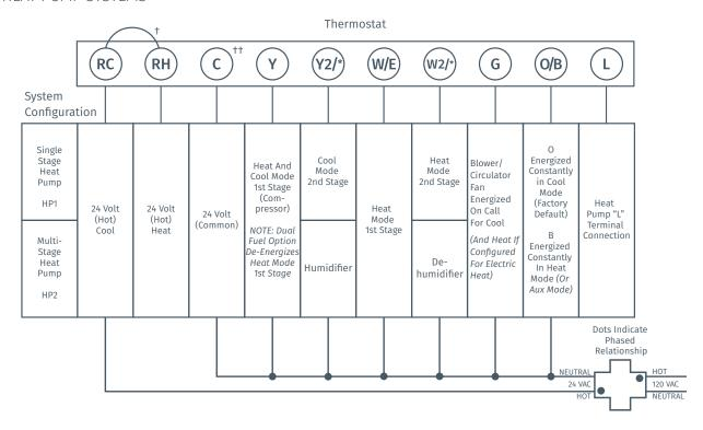
$^{\scriptscriptstyle \dagger}$  Internal jumper between RC and RH, located on back of thermostat.
