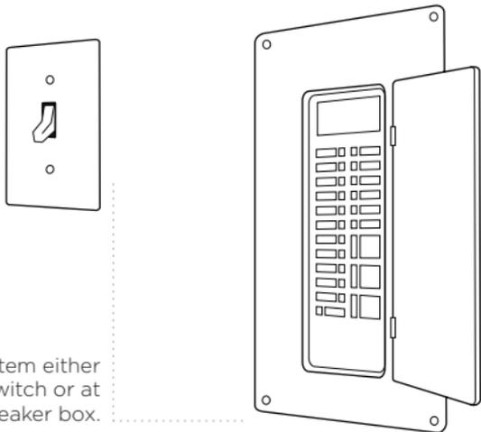
Power off your system either using the master switch or at the circuit breaker box.
