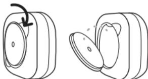
..... To access the battery, pop the remote sensor back cover off using the ridges provided.
