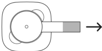
Stand in front of your ecobee3 and pull the plastic tab on the remote sensor to automatically pair it with your thermostat.
