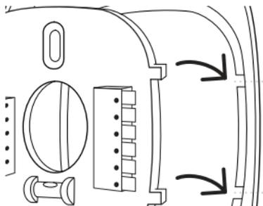
Insert the back plate using the tabs on the right as a guide. It will snap into place when correctly inserted.
