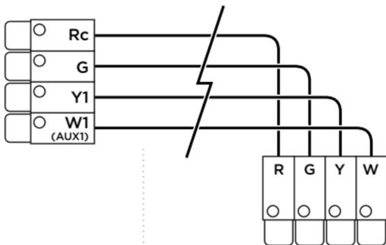
Wires coming out the wall and connecting to HVAC equipment
